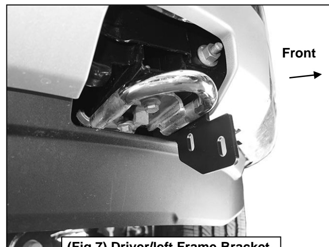
(Fig 7) Driver/left Frame Bracket installed with tow hook
